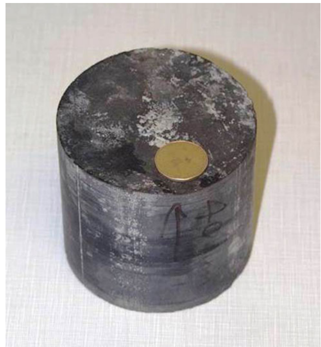
Fig. 1.17 Examples of typical core from a petroleum exploration hole
