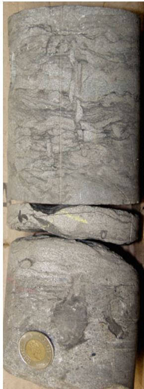
Fig. 2.24 Example of trace fossils in a drill core, showing how well these features can be seen. They include Skolithos (top) and Rosellia (bottom)
