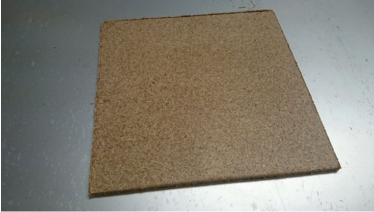
Fig. 3.3 Binding agent-free building boards made of Miscanthus
