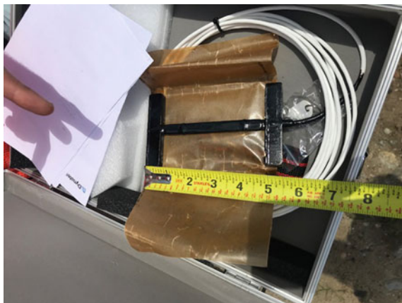
Fig. 2 Dynatest wheatstone bridge connection sensor
