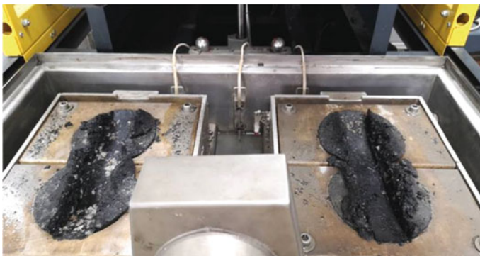
Fig. 4 Hamburg wheel track test samples after the test
