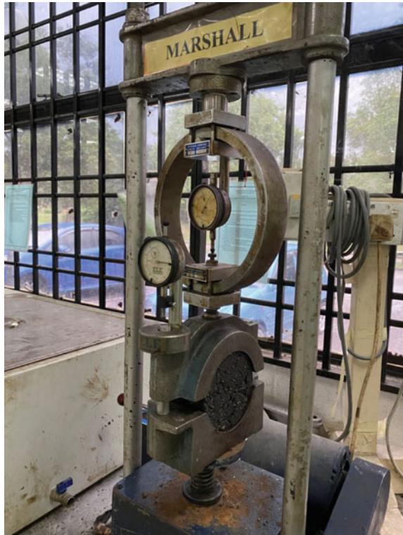
Fig. 3 Universal compression machine with Marshall loading fixture
