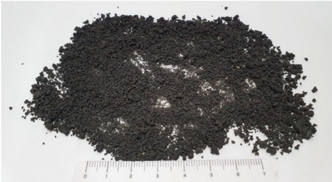
Fig. 8 Solid rubber particles recovered from extracted binder
