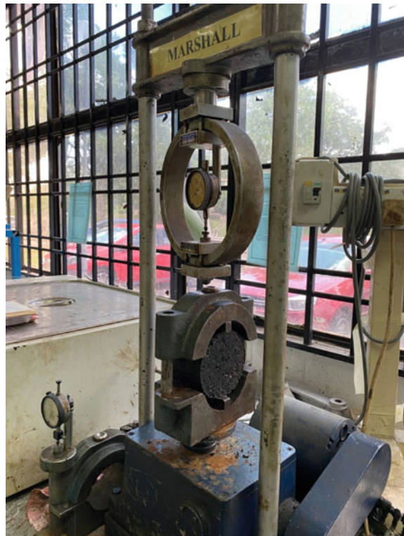
Fig. 4 Universal compression machine with ITS fixture
