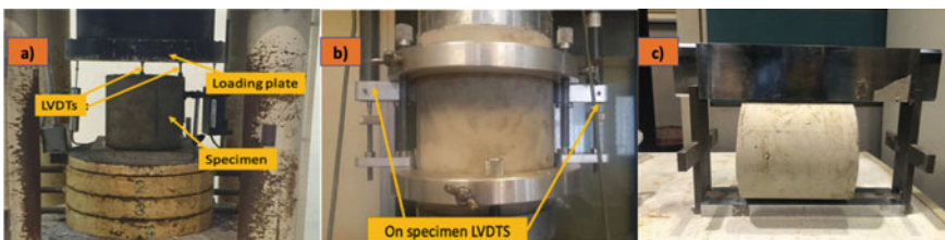
Fig. 4 Testing setup: a unconfined compression test; b modulus of elasticity test; c splitting tensile test
