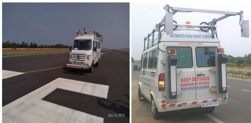
Fig. 4 Automated Road Survey System (ARSS) used for survey of Airfield Pavements
