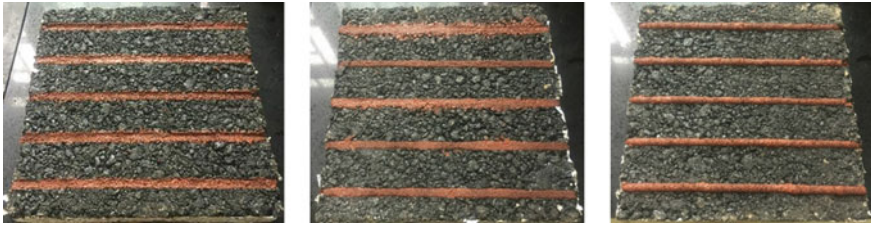
Fig. 3 Grooving filled elastomer specimen plates
