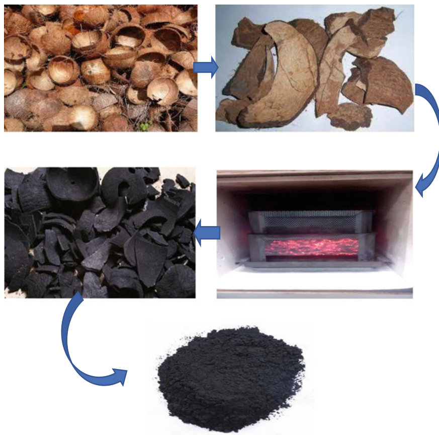
Fig. 2 The method of preparation of coconut char
