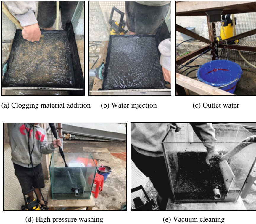
Fig. 1 Schematic diagram of procedure for laboratory clogging tests
