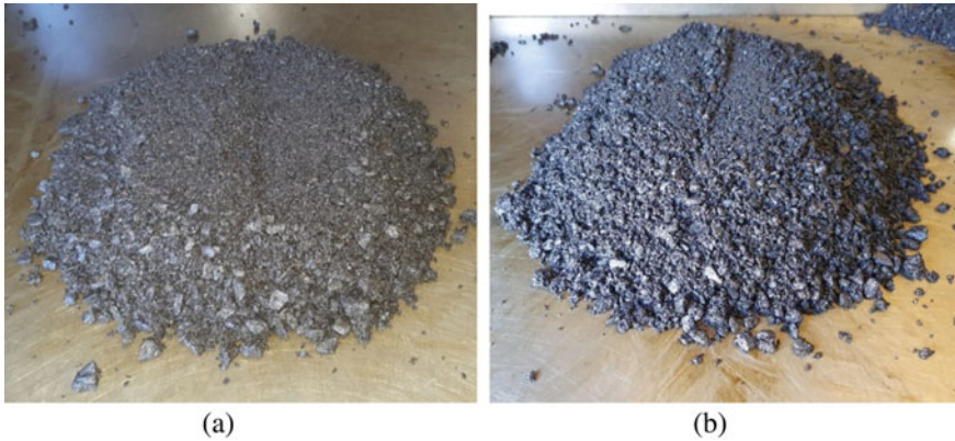
Fig. 9 Bulk asphalt samples with a 5.5% and b 7.0% binder content, both with 15% crumb rubber dosage
