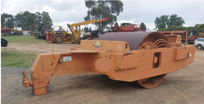
Fig. 3 Example 15 tonne vibrating steel drum roller
