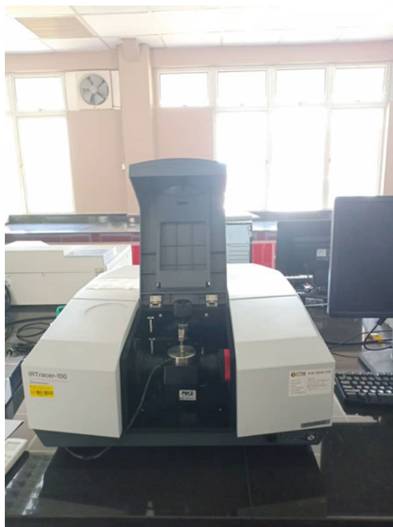
Fig. 4 Fourier transformation Infrared (FTIR)
