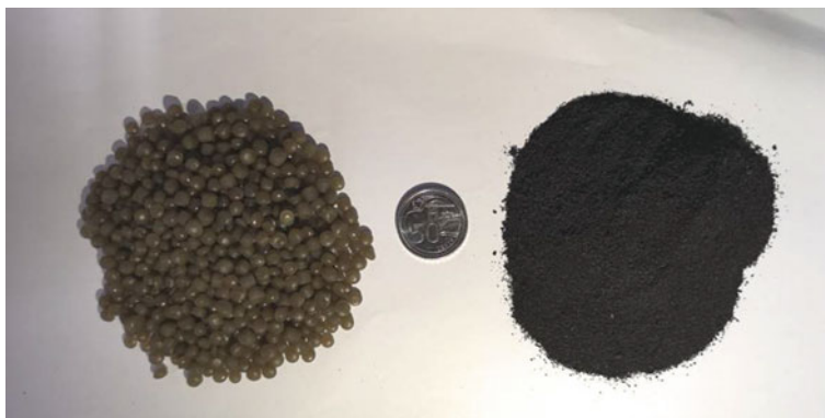
Fig. 1 Processed LDPE (left) and granulated crumb rubber (right)
