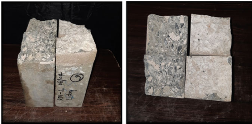
Fig. 7 Typical view of failure in repaired beams of substrate concrete
