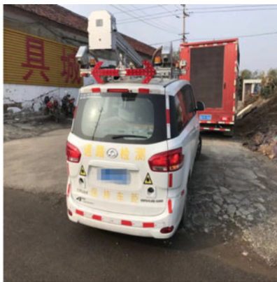
(a) Smartphone with APP (b) Multifunctional road condition detection vehicle
