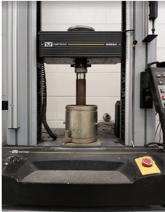
Fig. 2 Performing standard CBR test using Instron machine
