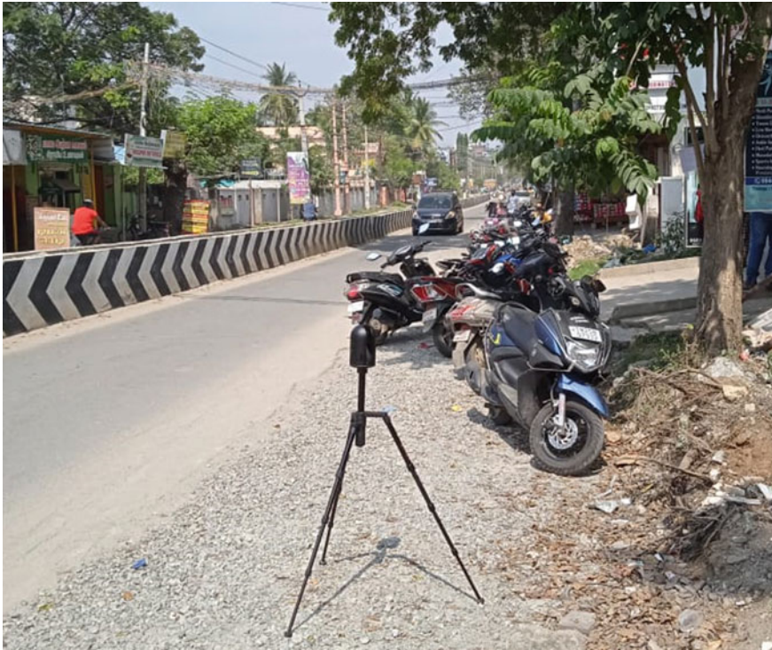
Fig. 3 LIDAR survey using Leica BLK 360 at Study stretch-1
