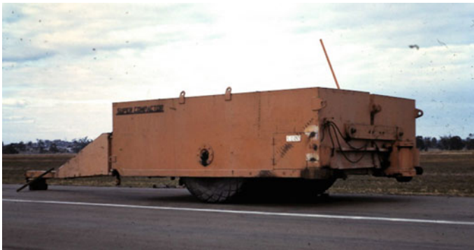
Fig. 2 Example 180 tonne Supercompactor
