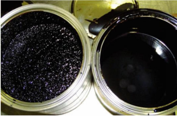
Fig. 7 Crumb rubber modified (left) and unmodified bitumen (right) binders
