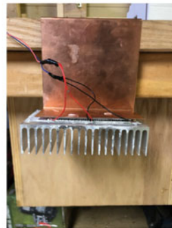
(b) Copper plate, TEGs, aluminium heat sink
