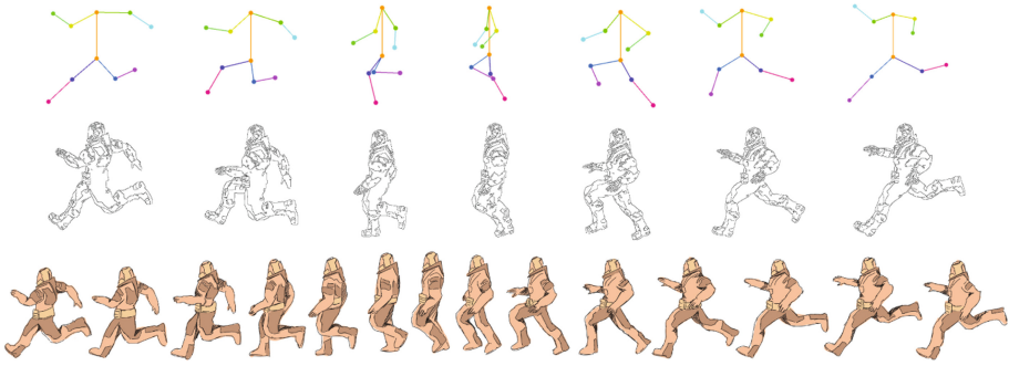
Fig. 1. Our program computes the joint angles of a set of key body joints to pose any 3D model. The posed model is toon-shaded and sketched over to help give a hand-drawn animation. Bottom row of frames were sketched and colored using the middle row reference keyframes.
