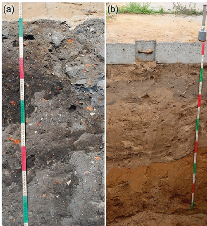
Fig. 5.2 Examples of urban soil profiles showing (a) the content of coarse fragments in an ‘urbic Technosol’ (an urban soil with significant artefact content) and (b) surface sealing in an ‘ekranic Technosol’ (an urban soil having hard material at the surface) (from Hulisz et al. 2018; used with permission from Springer)
