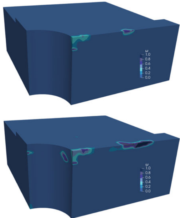
Fig. 3 Damage initiation (top) and propagation (bottom) within the second cycle, visualized in the reference configuration
