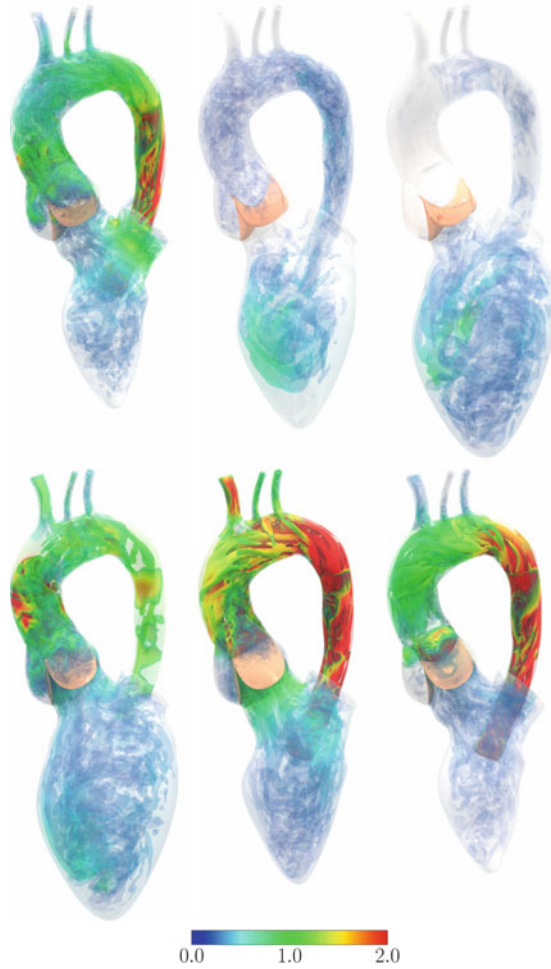
Fig. 4 Isosurfaces corresponding to a positive value of the second invariant of the velocity gradient tensor, colored by the velocity magnitude (m/s). The frames are for the same instants as in Fig. 2
