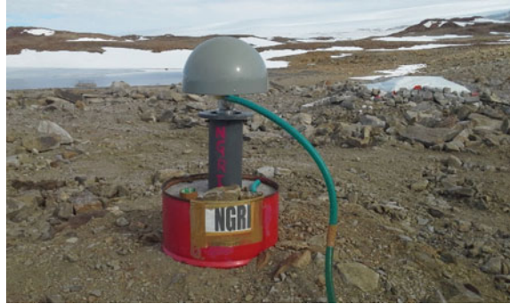
Fig. 4 The top panel shows the permanent G.P.S. antenna installed at Maitri. The lower panel shows the site velocity (observed) estimated from GPS measurements at Maitri and other Antarctica sites. Red vectors are the predicted site motion at these sites from the estimated pole location
