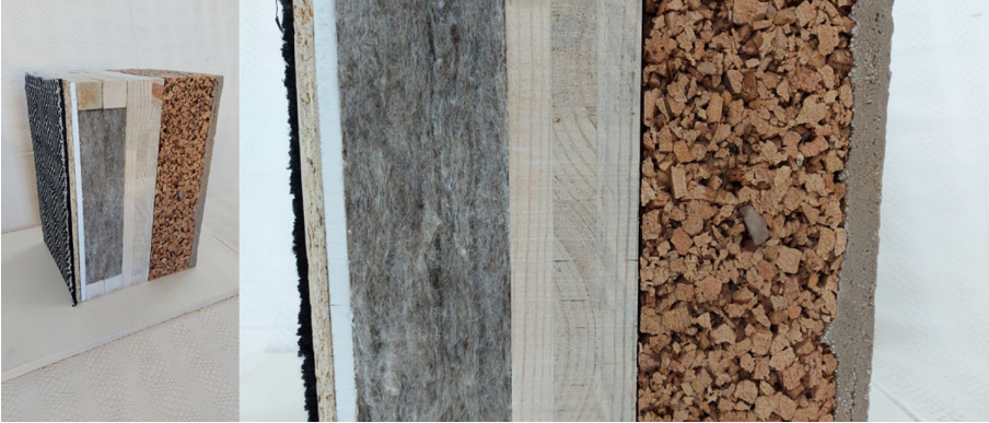
Fig. 13. Stratigraphy made of (from inside to outside): fine fabrics, wood panel, sheep's wool, 3-layer CLT, cork, natural plaster.
