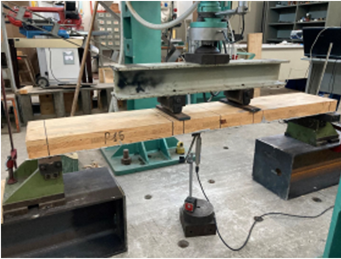
Fig. 9. Bending test on CLT panels.
