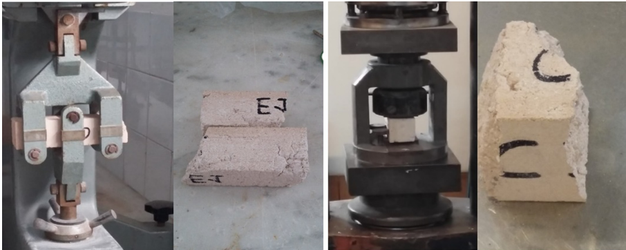
Fig. 3. Bending test (left) and compression test (right) on lime-plaster with natural fibres.
