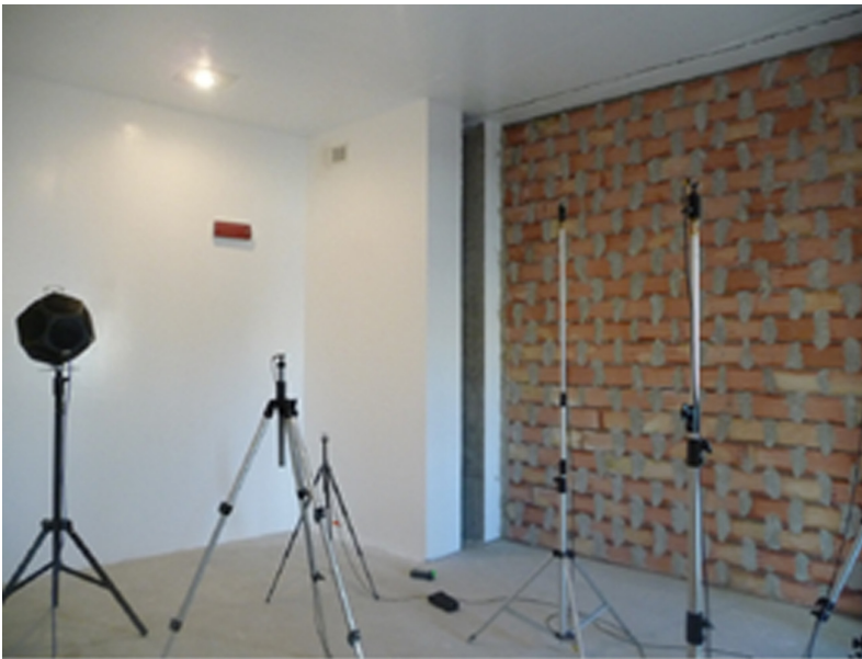
Fig. 10. Acoustic measurements on clay-brick masonry.
