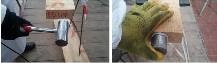
Fig. 2. Non-destructive sonic testing on Sardinian Maritime Pine boards.
