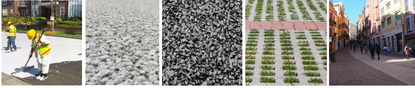
Fig. 2. Different types of “cool pavements”: colored, porous (concrete and asphalt), green and stone pavements (Color figure online).
