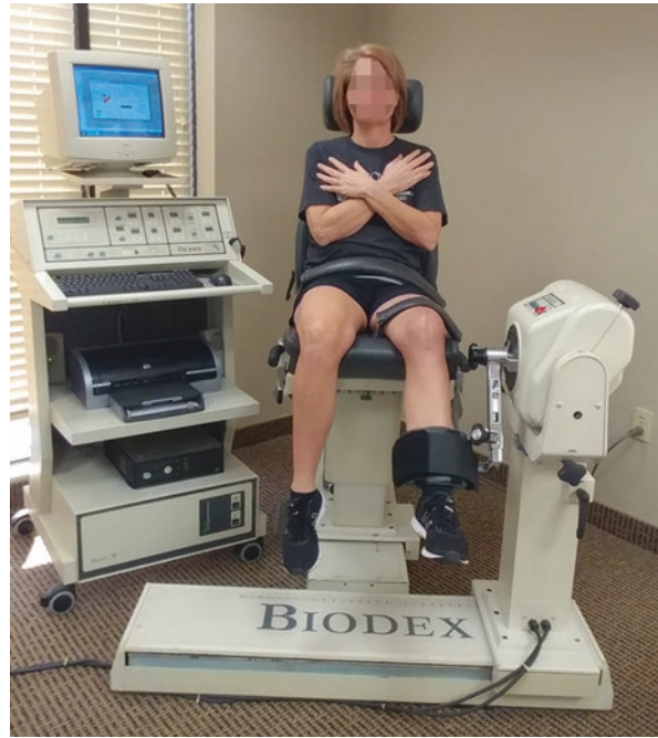
Fig. 7.1 Biodex test setup for isometric evaluation of quadriceps and hamstring muscle strength
