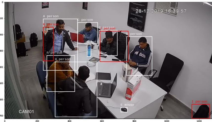
Fig. 5. Office scene with true (white bounding box) and false positive (red bounding box) object detection. Ids of persons will be used in text below (video source YouTube). (Color figure online)
