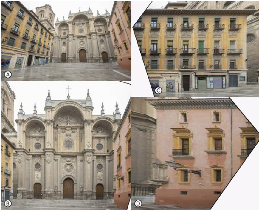
Fig. 14 Real example of the rectification of a photograph of the façade of the Granada Cathedral. a Original image, b rectified cathedral façade, c rectified left façade and d rectified right façade
