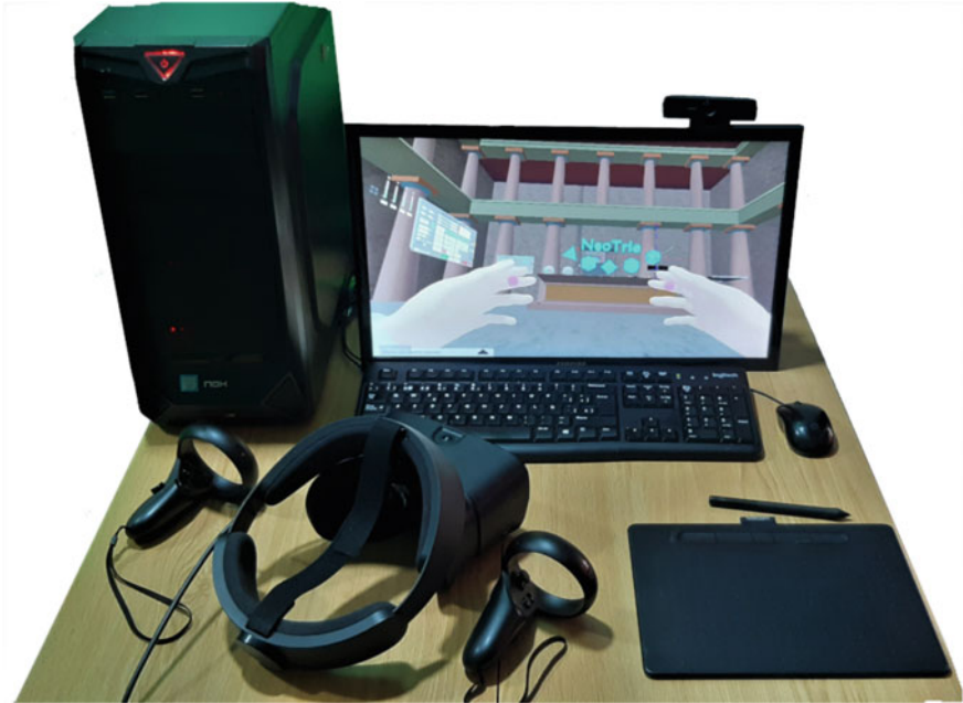
Fig. 3 Gaming PC, Oculus Rift-S, and digital tablet Wacom used by the teacher
