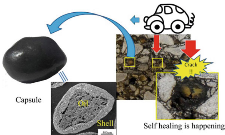
Fig. 21 Working mechanism of self-healing of asphalt mixture by the action of encapsulated rejuvenators containing sunflower oil as a rejuvenating agent (Reproduced from Garcia et al. [62])
