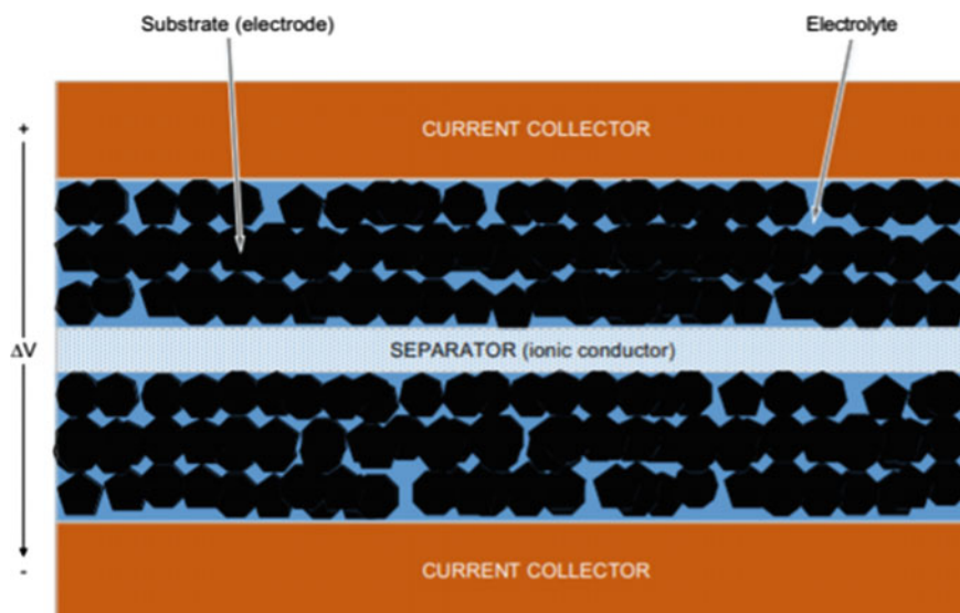
Fig. 5 Symmetric supercapacitor schematic diagram. (Reprinted with permission of [34])
