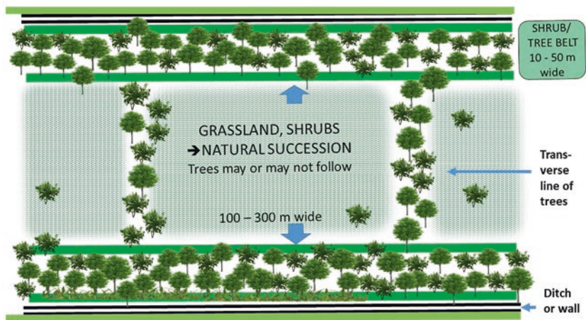
Fig. 5.2 Connective hydrologic module. (Note: Twin greenbelts (planted shrubs and trees) with area of natural succession between them)
