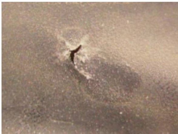
Fig. 2 Shell damage by localized pressure, with signs of peripheral stress
