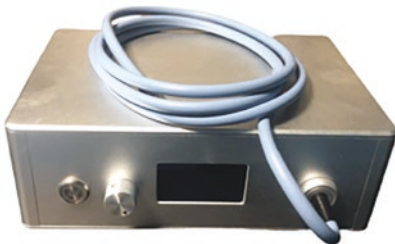
Fig. 33 Light source (LED) with fibre-optic cable in situ
