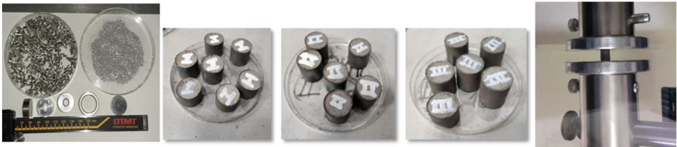
Fig. 8.2 Original of the AA7075 chip morphology as received from the company and atomized size, green compact just before sinter-forging operation followed by mechanical testing
