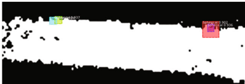
Fig. 7.2 Sample image from mask R-CNN implementation of porosity determination
