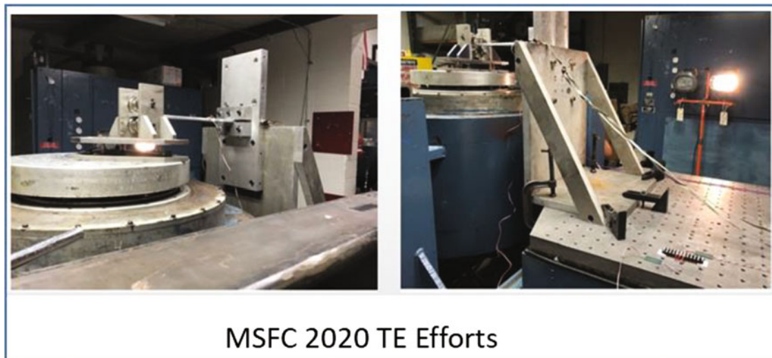
Fig. 13.2 Forced vibration test article and setup
