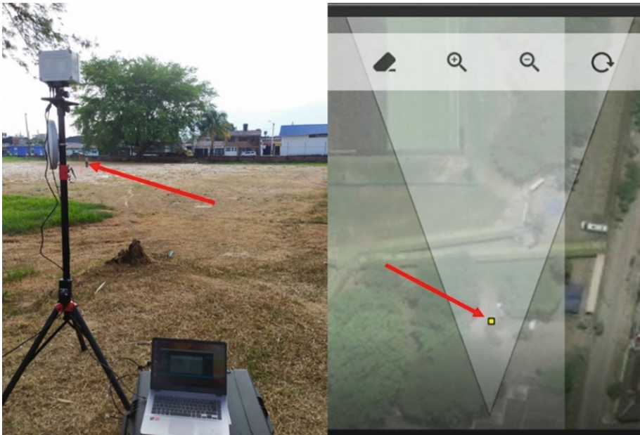
Fig. 7. Outdoor test protocol: the graphical user interface software shows the detection of a person who was walking in the radial direction to the radar.
