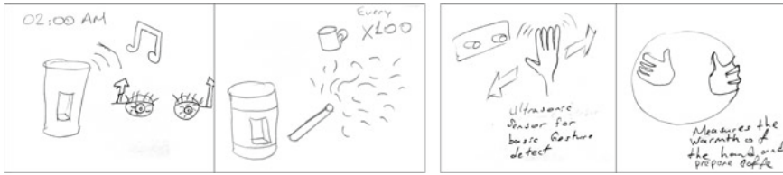
Fig. 9 Left: Explorations of user-product interactions for a coffee machine in Phase 1. Right: Explorations of new types of user-product interaction in Phase 4
