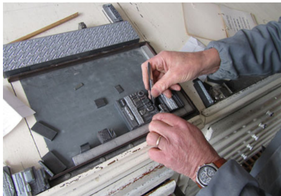
Fig. 7 The hands of printmaker Álvaro da Silva Gomes composing text (using movable types) for the intended label ( images source the author )
