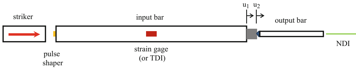
Fig. 11.1 A Kolsky bar used for high rate indentation
