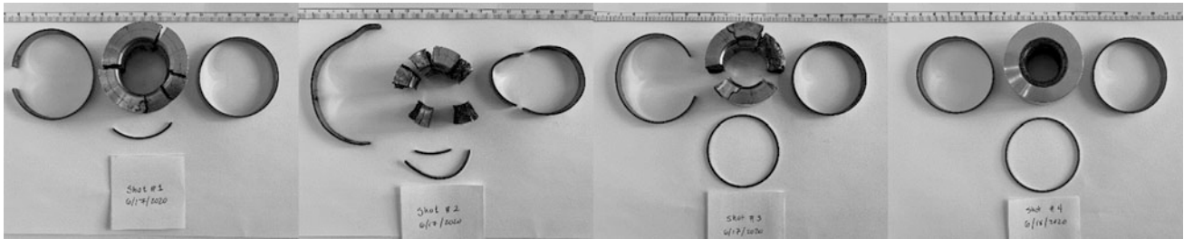
Fig. 15.4 Results of our first proof-of-concept tests. The drivers fractured in three of four cases
