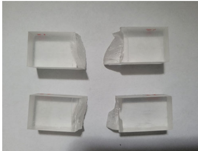
Fig. 14.5 Epoxy samples after impact from prototype loading device
