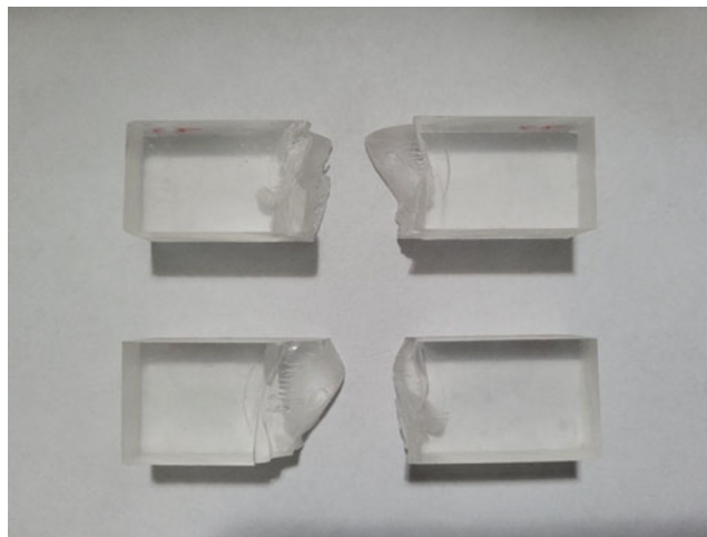
Fig. 14.4 Epoxy samples after impact from control loading device
