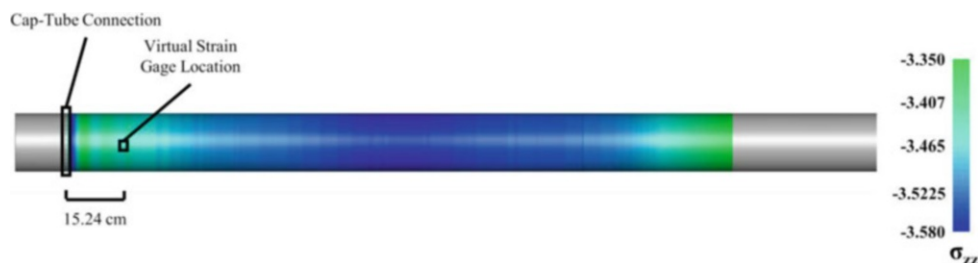
Fig. 2.5 Normal stress in the axial direction is shown 0.8 ms into the simulation. Elements having stress in the range of -3.58 to -3.35 MPa are shown in color. Elements with the axial stress outside that range are shown in grey
