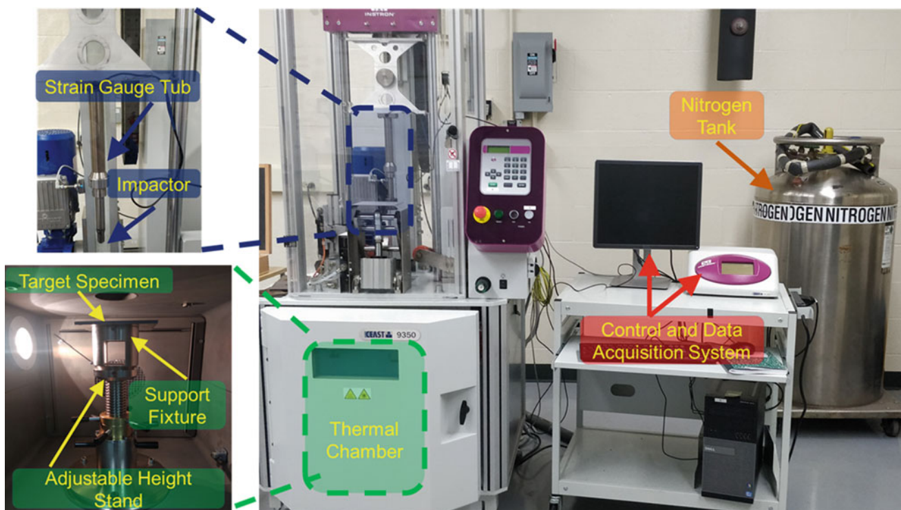
Fig. 4.2 Instron CEAST 9350 drop tower testing machine
