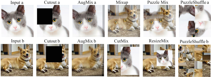
Fig. 2. A visual comparison of Cutout [1], AugMix [9], Mixup [28], CutMix [27], ResizeMix [19], Puzzle Mix [12], and our PuzzleShuffle
