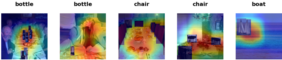
Fig. 4. Images from the Pascal VOC where the trained CNN network could not focus on target objects. Our method identifies some classes (i.a. ‘bottle’, ‘chair’, ‘boat’) where the model learned spurious correlations. Closer analysis shows that in this dataset, images in category ‘bottle’ also present people and/or tables.
