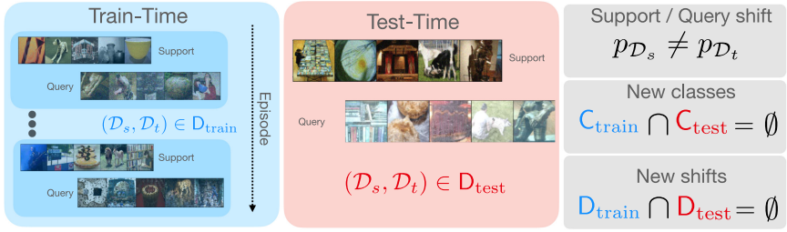
Fig. 2. During meta-learning (Train-Time), each episode contains a support and a query set sampled from different distributions (for instance, illustrated by noise and contrasts as in Fig. 1(b)) from a set of training domains ( \mathcal{D}_{\text{train}} ), reflecting a situation that may potentially occurs at test-time. When deployed, the FSL algorithm using a trained backbone is fed with a support set sampled from new classes. As the algorithm is subject to infer continuously on data subject to shift (Test-Time), we evaluate the algorithm on data with an unknown shift ( \mathcal{D}_{\text{test}} ). Importantly, both classes ( \mathcal{C}_{\text{train}} \cap \mathcal{C}_{\text{test}} = \emptyset ) and shifts ( \mathcal{D}_{\text{train}} \cap \mathcal{D}_{\text{test}} = \emptyset ) are not seen during training, making the FSQS a challenging problem of generalization.
