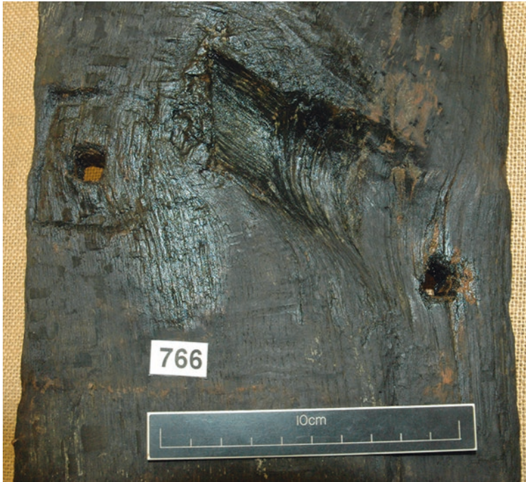
Fig. 1.3 Inboard face of Newport Ship hull plank 766 showing pruned side branch encapsulated in later tree growth. A rare example of direct proof of woodland management. (Photo Newport Museum and Heritage Service)
