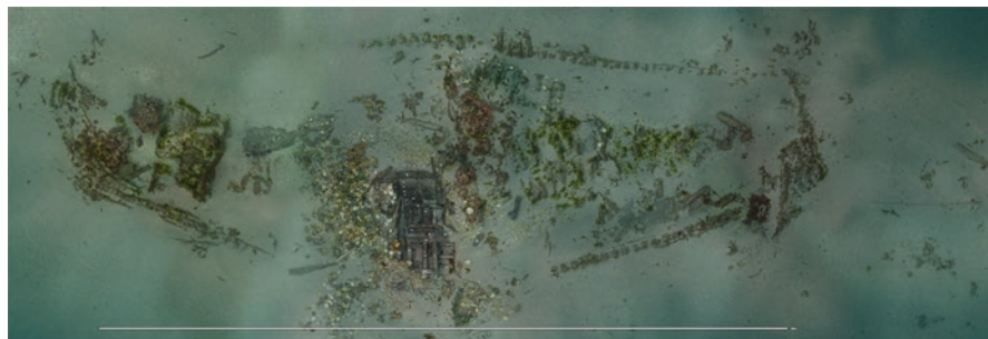
Fig. 3.3 Photogrammetry of the Ribadeo's galleon site. We can see the wreck, during 2019 excavation season with the bow to the right bearing North. The upper frames in fact are beams from the first deck. Really frames are seeing on the low right of the picture. The excavated central area is surrounded by bulkheads. The white scale is 30 m
