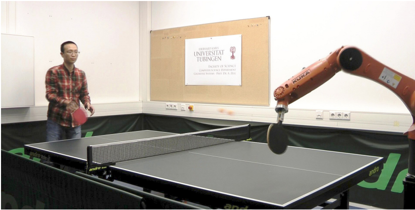
Fig. 1. Playing with our KUKA table tennis robot. A wearable IMU is mounted at the bottom of the player’s racket handle. The quaternion value q_{IMU} streamed from it, is defined as the racket orientation in the IMU frame. One of the stationary cameras fixed on the ceiling is used to capture the human player movements from above (Fig. 2 left). By fusing the images with IMU signals, we can take them as inputs and regress the 3D racket position robustly with the proposed approach. The camera and the IMU are synchronized with a software trigger.
