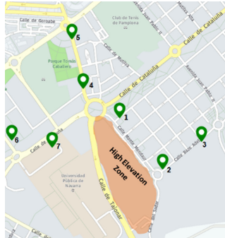
Fig. 5. SigFox measurements results. Green: No packet losses. Yellow: some packet losses. Red: All packets lost (Color figure online).
