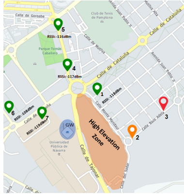
Fig. 4. LoRaWAN measurements results. Green: No packet losses. Yellow: some packet losses. Red: All packets lost (Color figure online).
