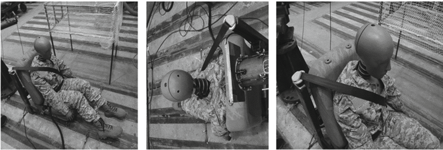
Fig. 5. Hybrid III 50 th Percentile Male Dummy – Position during the test.
