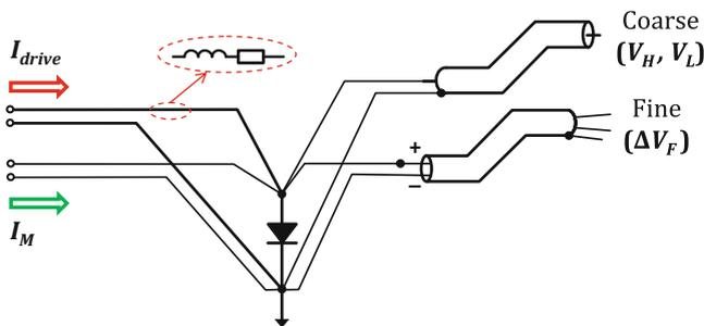
Fig. 5.6 Thermal transient measurement of a diode, powering, and sensing arrangement shown
