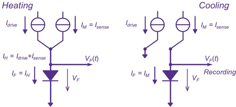
**Fig. 5.10** Practical realization of the diode measurement scheme: (a) applying heating current; (b) cooling at constant measurement current
