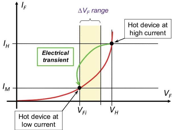
**Fig. 5.13** Thermal (cooling) transient of the diode at constant measurement current shown in its  $I-V$  characteristics. This chart is an enlarged portion of Fig. 6.1
