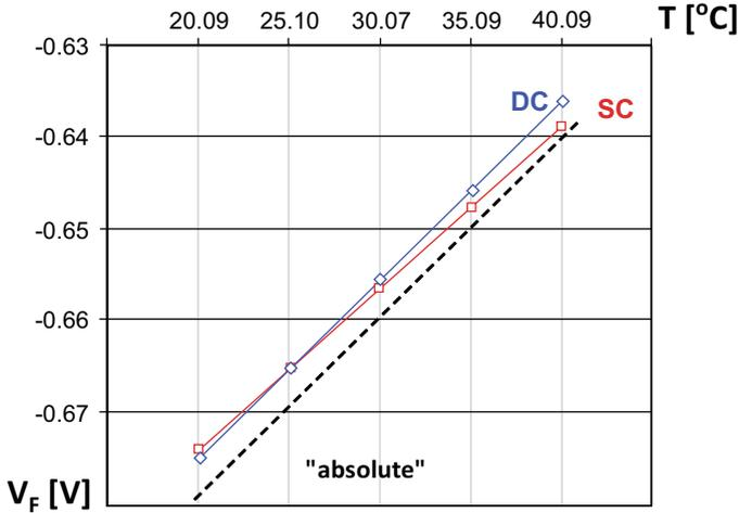
Fig. 5.22 Example on the absolute calibration error
