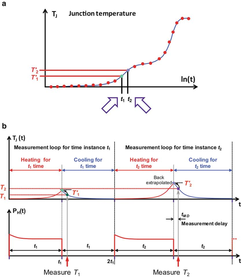
Fig. 5.17 The principle of the JEDEC JESD51-1 dynamic test method: (b) the series of heating pulses and corresponding temperature responses, (a) heating curve composed of individual temperature values measured at the end of the heating pulses
