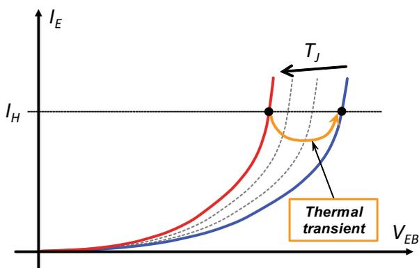
transient is very fast, just a few  $\mu\text{s}$ , which is near to the slew rate of the power sources in the best transient testers.
