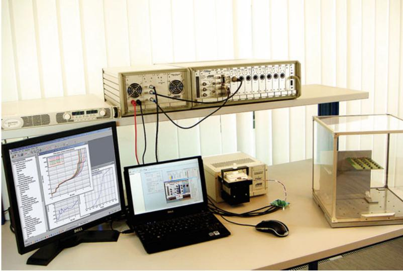
**Fig. 5.15** Typical thermal transient measurement arrangement: test equipment, thermostat for TSP calibration or to be used as a cold plate, natural convection test environment, and PC with measurement control and data processing software
