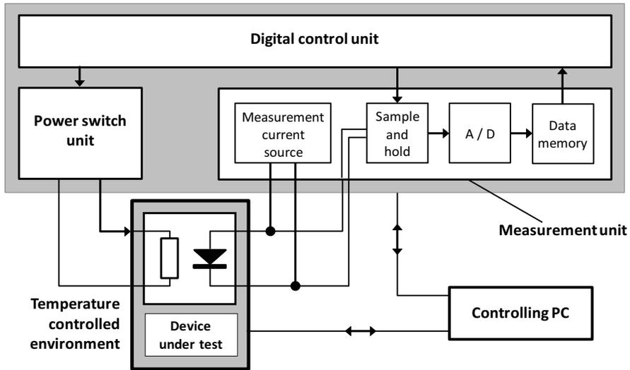
Fig. 5.2 The general scheme of the tester and test environment
