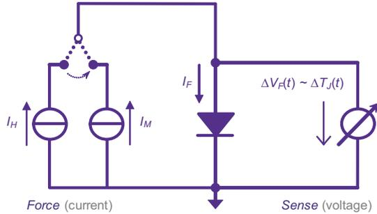
The  $I_H$  heating current is provided as the sum of the currents of the  $I_{drive}$  and  $I_{sense}$  current sources; thus, in the heating period, both currents are applied on the device for an equalization time of appropriate duration (Fig. 5.10a). When the device reaches the “hot” steady state, the drive current is switched off.
