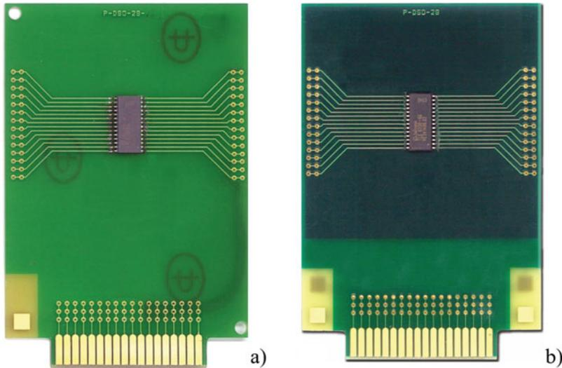
**Fig. 5.3** Integrated circuit in DIP package on standard printed boards as defined in the JEDEC JESD51 set of standards, (a) worst-case cooling with one patterned copper layer (b) with two solid internal copper layers for enhanced cooling. Separated force and sense traces can be observed
