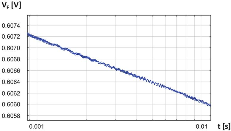
**Fig. 5.26** High-frequency interference from an external source on a measured thermal signal
