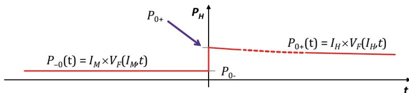
**Fig. 5.16** Power change before and during the heating measurement on a diode
