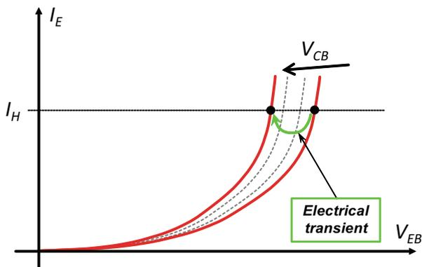
**Fig. 5.20** Thermal transient of a transistor after switching  $V_{CB}$  from high to low voltage
