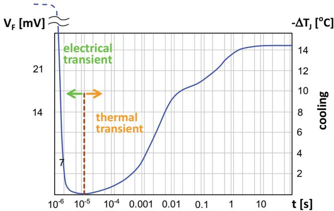
**Fig. 5.14** Recorded transient of an actual diode, scaled in voltage (on the left) and in temperature (on the right)
