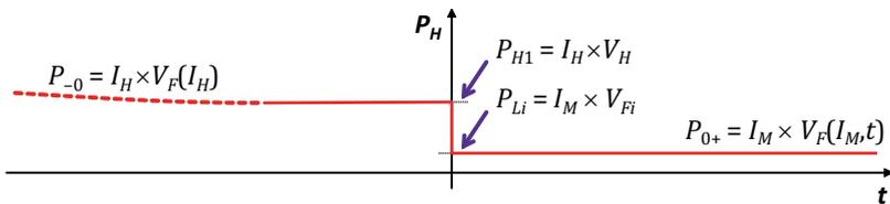
**Fig. 5.11** Power change before and during the cooling measurement on a diode
