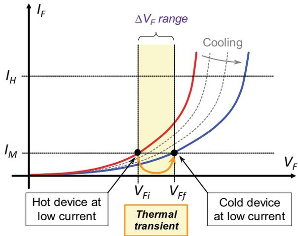
The measurement channel has to be capable to record the complete transit of the  $V_F$  voltage between its hot and cold value, in an appropriate “fine” measurement range covering  $\Delta V_F$ . Still, the fast travel of the signal during the electric transient is not recorded always in its entirety; the signal may jump into the “fine” measurement range from an “out of range” condition. The necessary  $\Delta V_F$  range of recording is highlighted in Figs. 5.12 and 5.13.
