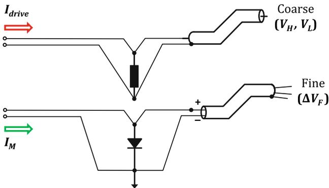
**Fig. 5.5** Thermal transient measurement of a thermal test vehicle with separated powering and sensing
