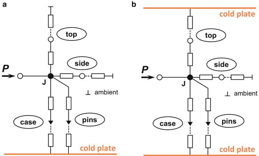
Fig. 5.21 Calibration of a component mounted on single and dual cold plate
