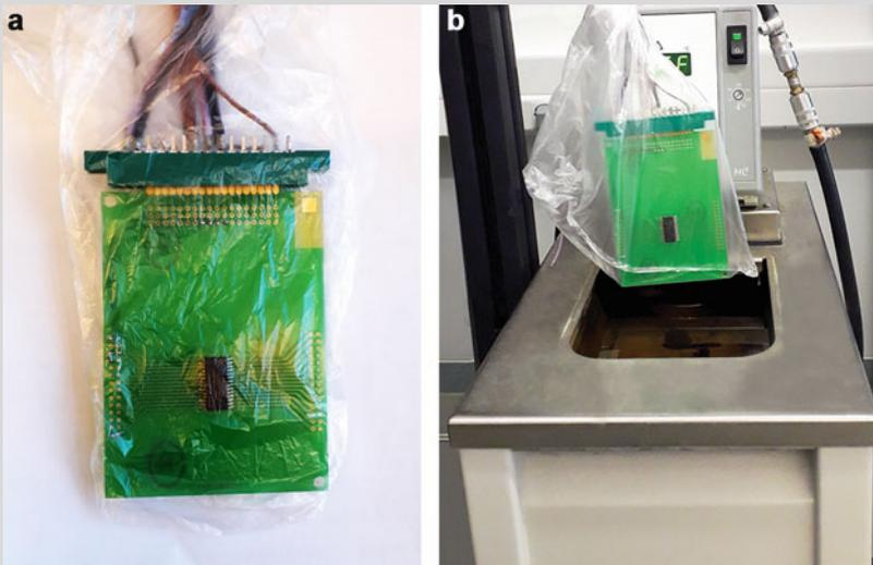
**Fig. 5.25** Water-filled liquid circulator with open vessel. Printed board placed in three plastic bags prepared for TSP calibration
