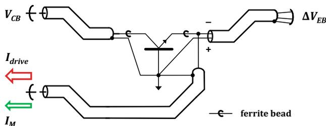
**Fig. 5.18** Measurement of a transistor in common base configuration
