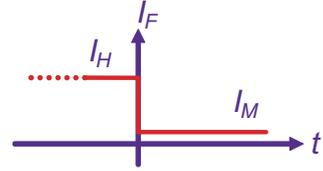
**Fig. 5.9** Diode measurement scheme as defined by the JESD51-1 standard
