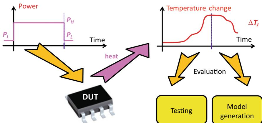
Fig. 5.1 Thermal transients in a system and their use for testing and modeling
