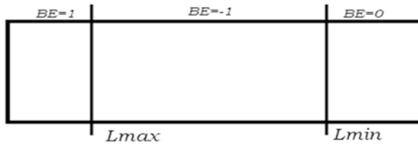
Fig. 3 Two buffer limits are marked in the WSN node
