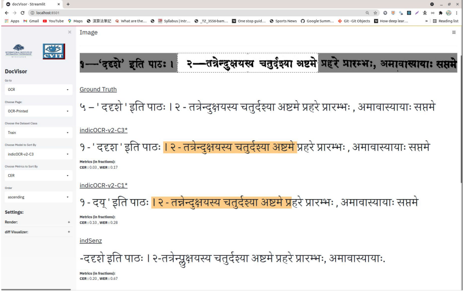
Fig. 8. OCR interface in DocVisor depicting the image-text alignment by leveraging the attention mechanism from the OCR architecture of Agam et al. [5]. Refer to Sect. 5. Notice that there are multiple (2) attention OCR models along with non-OCR models that can be loaded in the OCR layout that allows the user to compare line level results of multiple models simultaneously.
