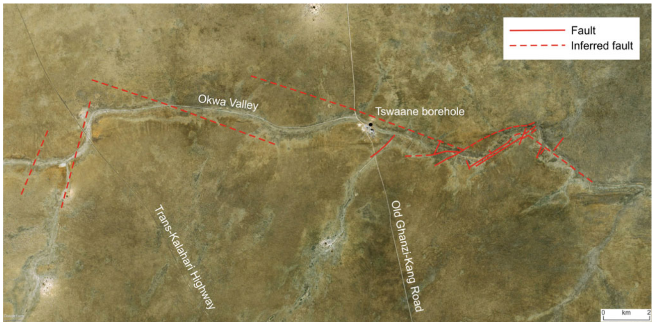
Fig. 11.12 Fault-controlled section of the Okwa Valley close to Tswaane borehole. Approximate positions of faults shown as red lines, dashed when inferred. Fault patterns redrawn after Aldiss and Carney (1992) and Ramokate et al. (2000)
