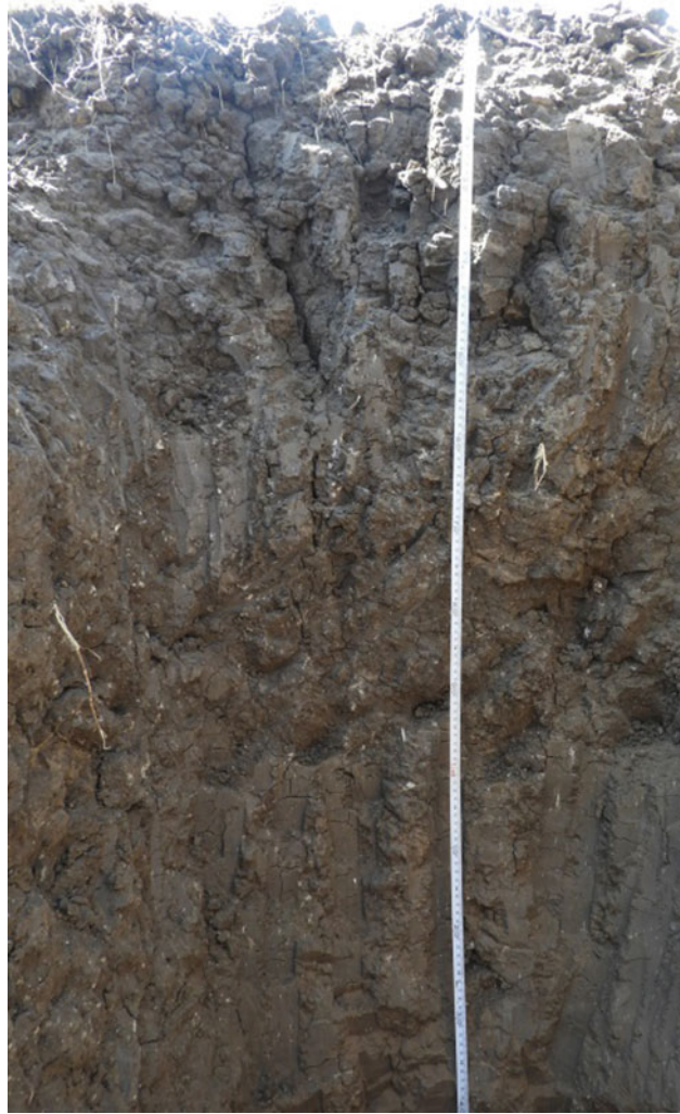
Fig. 19.16 Pellic Vertisol (Calcaric) developed on basalt in a sedimentary lowland, Serowe. Depth is >120 cm
