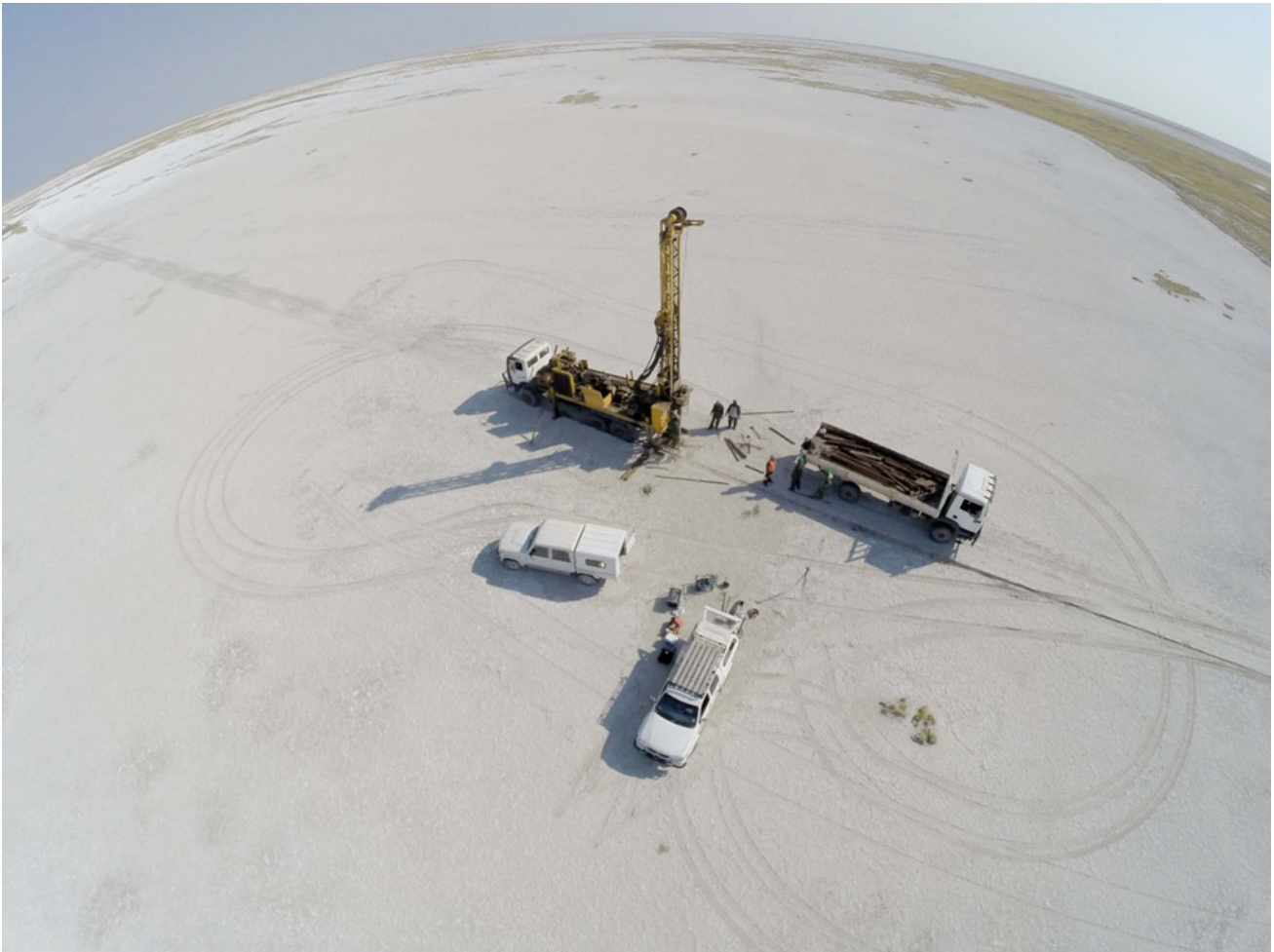
Fig. 5.5 A team from the Geoscience Institute of Botswana extract lake-bed cores from Ntwetwe pan for terrestrial proxy analysis to reconstruct lake-level fluctuation and past climate change
