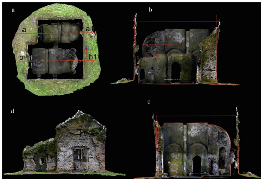
Fig. 2 Temple Nizhnaya Dranda according to photogrammetry data: a —plan; b —view of the south wall along the section of line aa1 ; c —view of the north wall along the section of line bb1 ; d —view of the western facade from the outside
