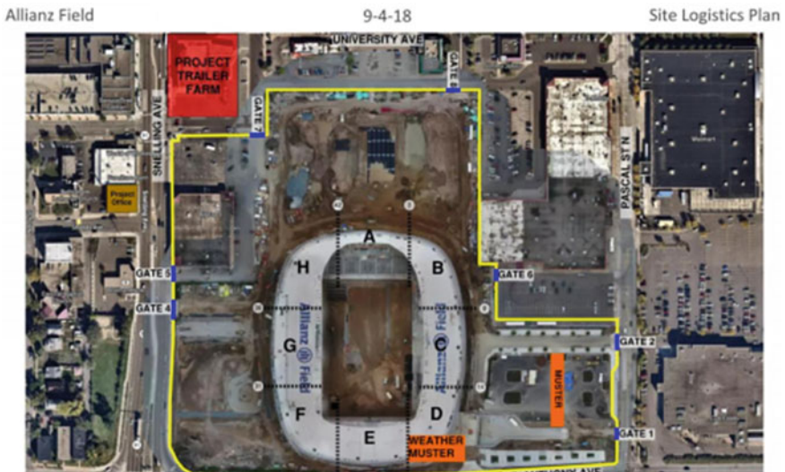
Fig. 4.10 A Case Study of Drones used for Overall Site Logistics Plan for Entire Project Team (Gibson & McManmon, 2018)
