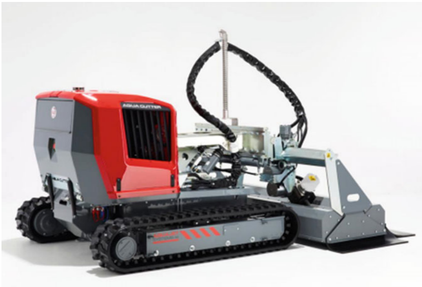
Fig. 7.7 Hydro-powered demolition robot (Ruggiero et al., 2016)
