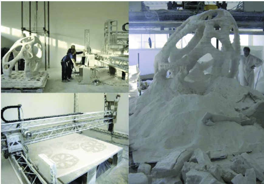
Fig. 6.5 D-shape printing technology (Hamad et al., 2018)
