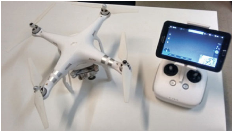
Fig. 4.14 DJI phantom 3 advanced with a tablet Samsung Galaxy Tab E 7 for display (Santos-de-Melo et al., 2017)
