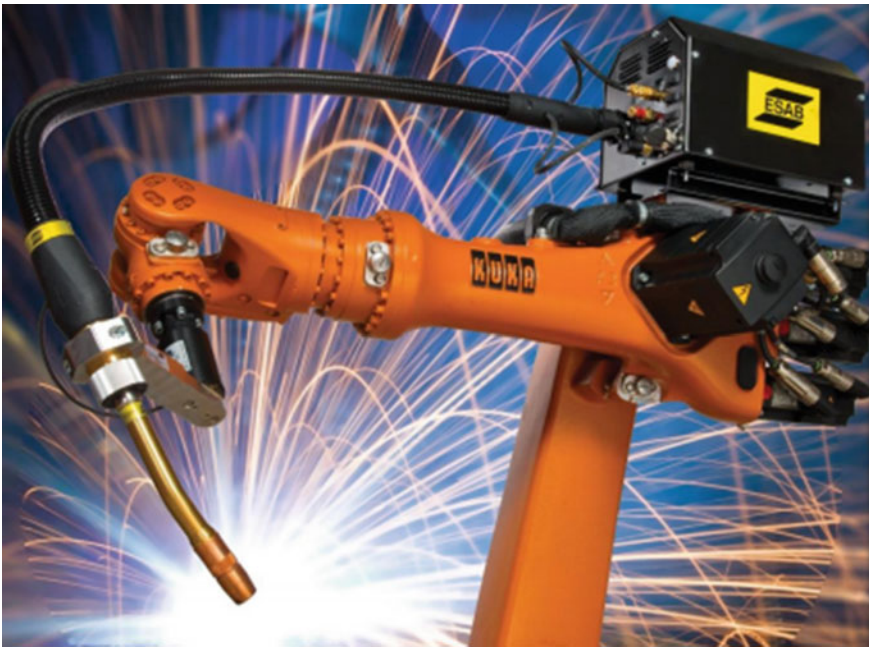
Fig. 7.11 Welding robot (Ruggiero et al., 2016)
