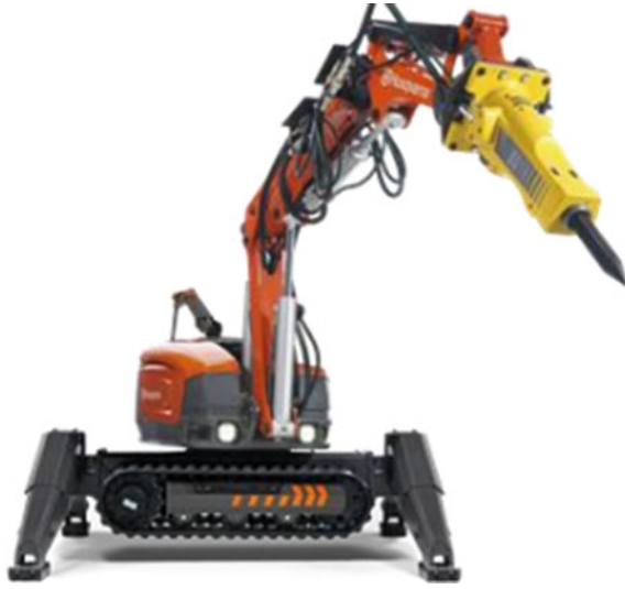
Fig. 7.6 Multi-tooled demolition robot (Ruggiero et al., 2016)
