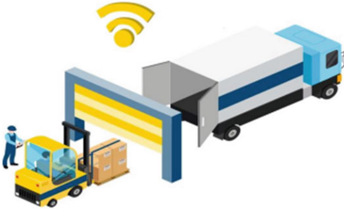
Fig. 8.9 Construction materials being identified and counted at construction site gate (Patil & Shelake, 2021)
