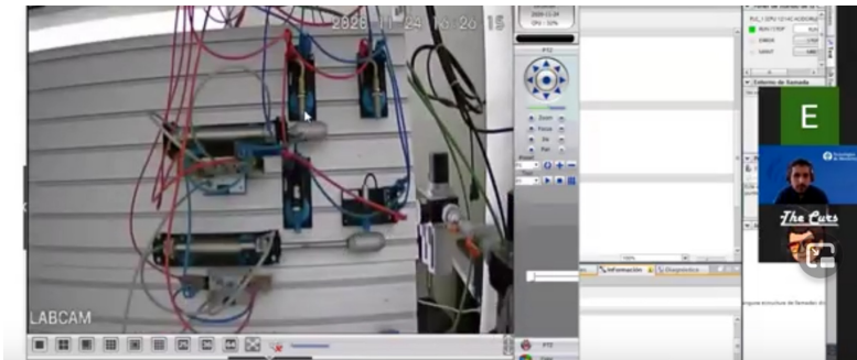
Fig. 1. Remote laboratory setup consisting of cylinders being controlled by PLCs. Remote desktop software and a webcam allowed to execute the code in real-time.
