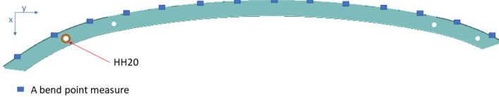
Fig. 1. Measurement points on the beam. The blue rectangles represent the different measurement points of the bend. Hole HH20 is the leftmost hole in the beam. (Color figure online)
