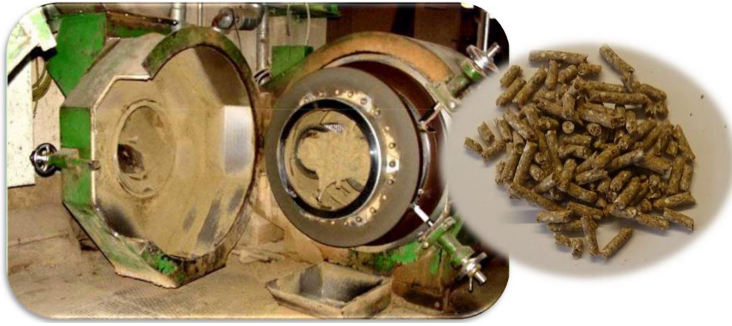
Fig. 2. Pellets after compaction in a press machine (Source: DVT, p.2)
