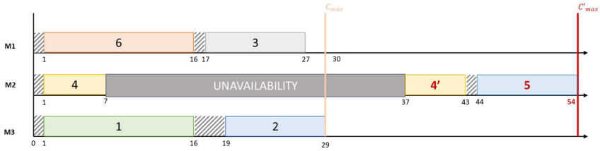
Fig. 3. Rescheduling example after machine unavailability with stability equal to 0
