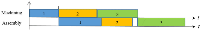
Fig. 3. Gantt chart of the “frame” schedule for the manufacture of components and assembly of products from them.
