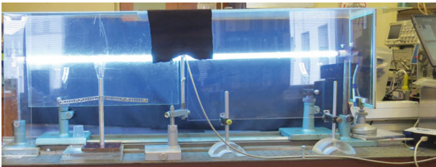
Fig. 3 Placement of a mercury lamp for experiments to measure the attenuation of radiation passing through the PTFE layers
