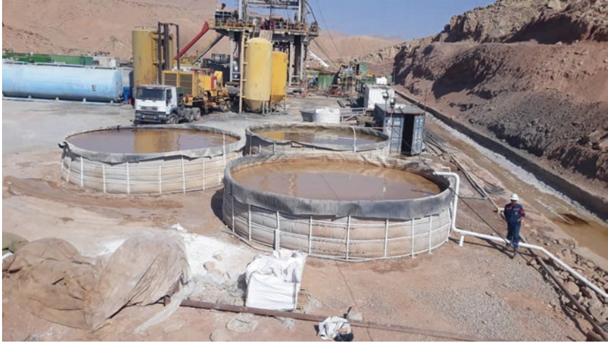
Fig. 4.4 Polyethylene cyclonic series of ponds mounted with iron structures. (Naft Sefid, Shushtar County, Khuzestan province, Iran, 2019)
