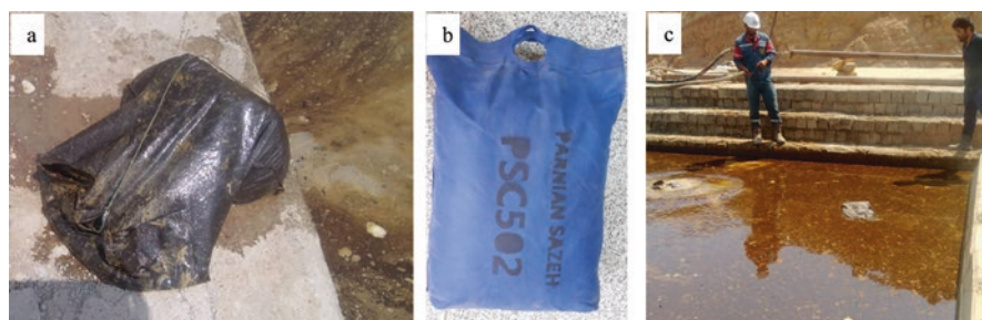
Fig. 4.6 Organic oil absorbent made by anaerobic thermal treatment of sugarcane bagasse coir (Naft Sefid, Shushtar County, Khuzestan province, Iran, 2019). (a) Absorbent after oil absorption is extracted out of the water; (b) clean absorbent before the oil absorption process; (c) the organic absorbent floats on the contaminated water and absorbs the oil pollution
