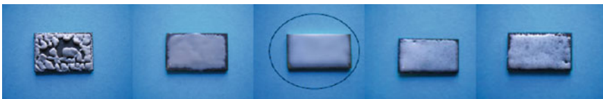
Fig. 2 Effect of different powder sizes on the compatibility between a glass–ceramic sealant (SACN) and a Crofer22APU stainless steel substrate. From left to right different SACN powders sizes: d < 20 \mu\text{m} , d = 20\text{--}38 \mu\text{m} , d = 38\text{--}75 \mu\text{m} , d = 75\text{--}106 \mu\text{m} and d > 106 \mu\text{m} [10]
