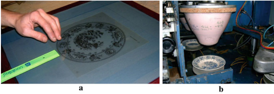
Fig. 20 Details of the pad printing process: a Steel screen ink impression step, b the silicone pad in the position after image printing on the ware (by courtesy of Faianças Primavera Company)
