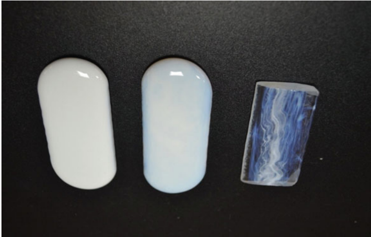
Fig. 8 From the right to the left: pattern of the annealed glass 2 (rightmost), annealed glass 3 (in the center of the figure) and pattern of the glass 3 heat treated at 1000 °C for 2 h (see also Fig. 6)
