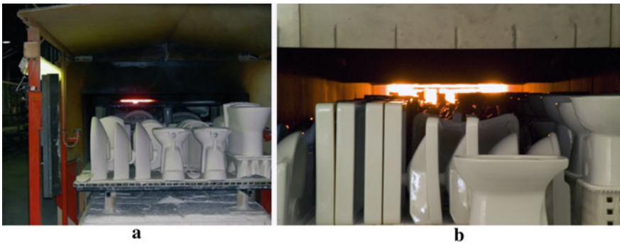
Fig. 14 Gas tunnel kiln for sanitaryware a kiln inlet, b kiln exit (by courtesy of Sanindusa Company)
