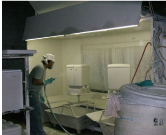
Fig. 13 Manual spray glazing of sanitaryware (by courtesy of Sanindusa Company)
