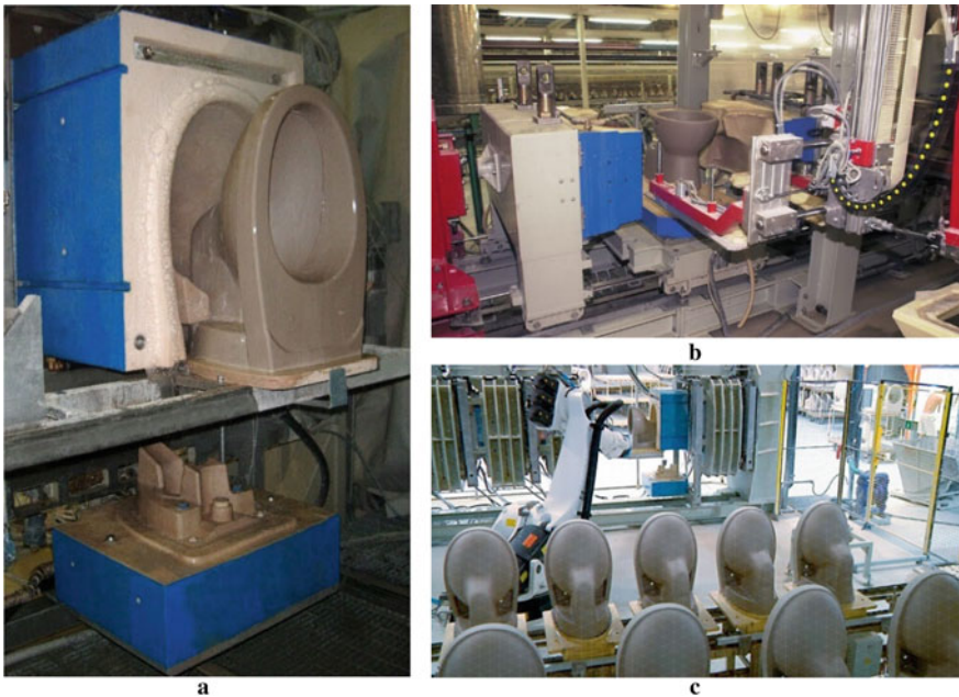
Fig. 11 WCs production; a resin mold, b hydraulic manipulator demolding, c general view of an automatic WCs line production (by courtesy of SACMI Company)
