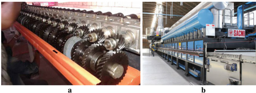
Fig. 9 Image of a gear drive system for a roller kiln movement (a), and photo of the exit in SACMI roller kiln single layer, for the ceramic tiles firing (b) (by courtesy of SACMI Company)
