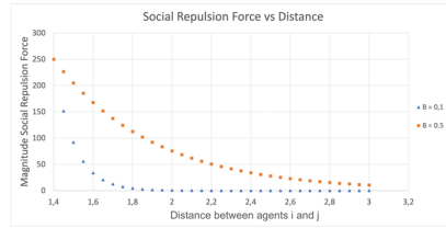
Fig. 4. Plot of social repulsion force f_{\text{social repulsion}} [N] vs distance between the passengers d_{ij} [m]. The blue graph is the social repulsion force of the baseline AATOM model (when agents are not physically distancing). The orange graph is the social repulsion force for the extended AATOM model where agents are physically distancing. (Color figure online)
