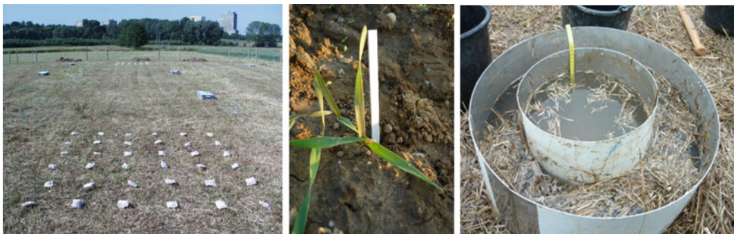
Fig. 3.7 Functional methods. Left: Litter-bag test with a single bag (inlet). Center: Bait-lamina test with single strips (with/without fed holes) individual strip (inlet). Right: Water-infiltration test. Photos J. Römcke
