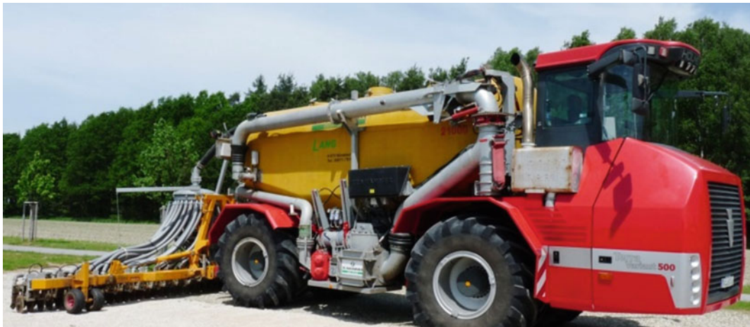
Fig. 2.5 Self-propelled Trac for transport and application/injection of liquid manure and digestate from biogas plants. Though rules for the prevention of soil compaction exist (e.g., Weyer and Boeddinghaus 2016),
