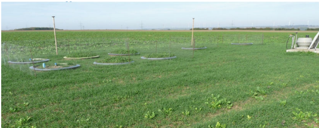
Fig. 3.4 Lysimeters embedded in a cropped field for agri-environmental monitoring of soil and groundwater pollution. On the right side there is the entry into the lysimeter cellar containing probes and samplers. Photo L. Mueller
