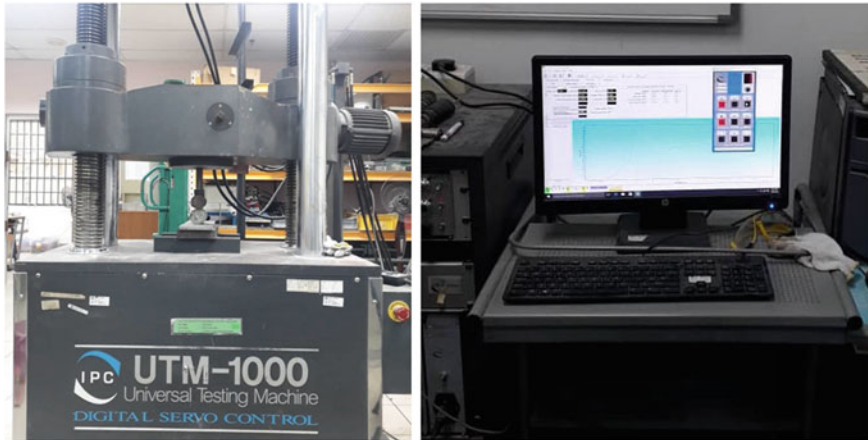
Fig. 14.5 Splitting Test, (a) IPC UTM-1000 Universal Testing Machine and (b) Computer to monitor and record the splitting tensile testing
