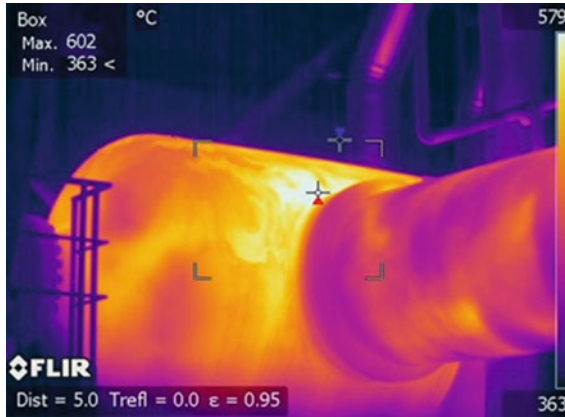
Fig. 11.2 Skin metal temperature survey from IR Thermography during the incident
