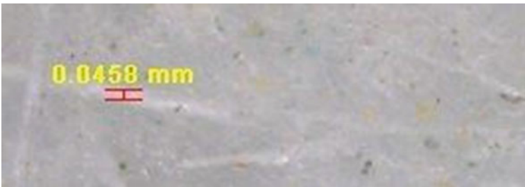
Fig. 20.9 -45^\circ crack initiation width
