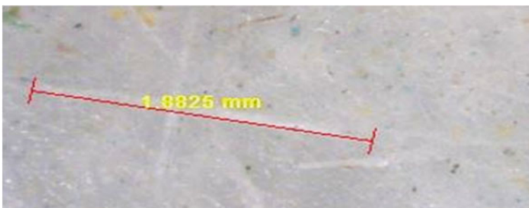
Fig. 20.7 +45° Crack initiation length
