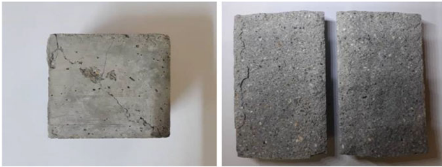
Fig. 14.7 Fractography surface of specimen: (a) Cube and (b) Cylinder
