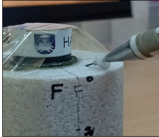
Fig. 16.4 Handling method of the pencil lead on surface of the granite
