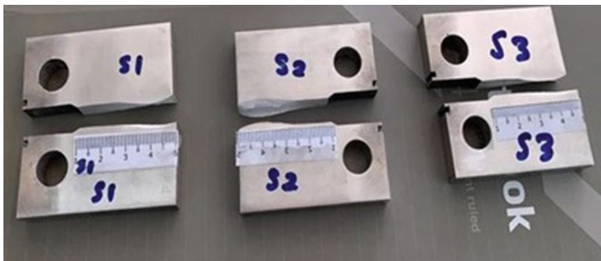
Fig. 12.9 Three samples of AZ31B CT with respective crack lengths
